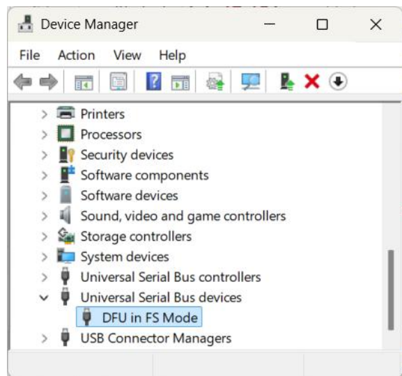
Fig. 10a a 10b: DCC-prog in DFU mode in Device Manager without and with the DFU driver installed
